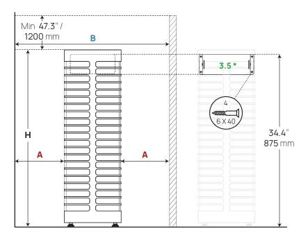
\* STEEL Mini 3.5 is attached to the wall with a special bracket See STEEL Mini 3.5 heater data in the table below.
